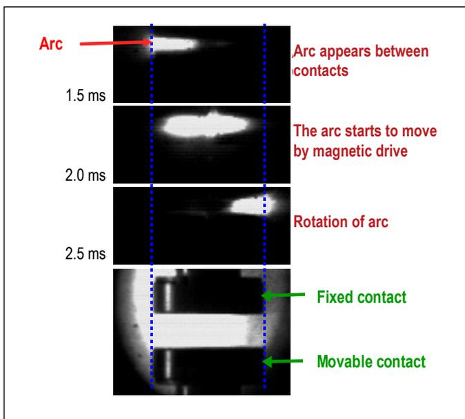
Figure 4 — The Arc Motion of Spiral Contacts
