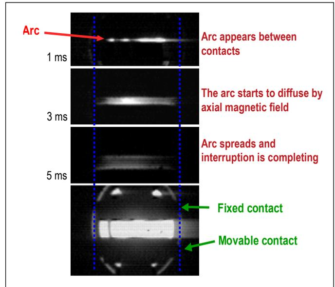
Figure 5 — The Arc Motion of AMF Contacts
