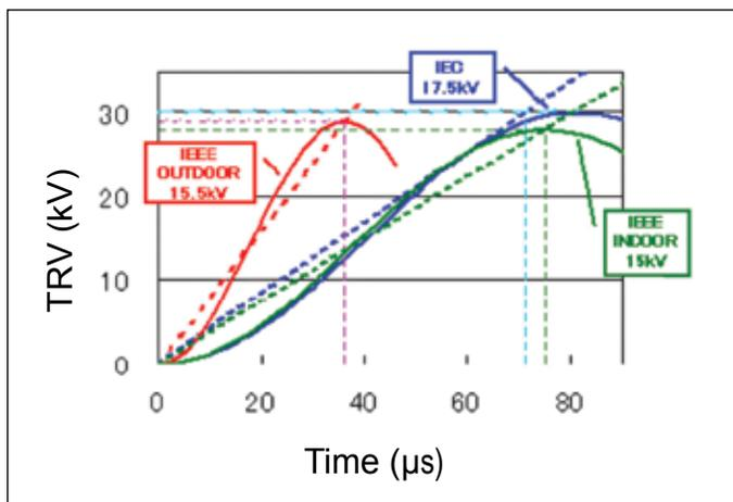
Figure 9 — TRV Waveform for 15-17.5 kV Breaker
