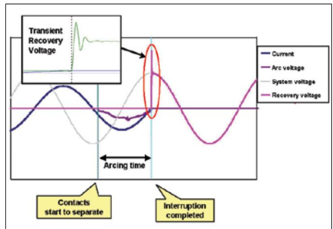
Figure 6 — Oscillograph During the Interruption
