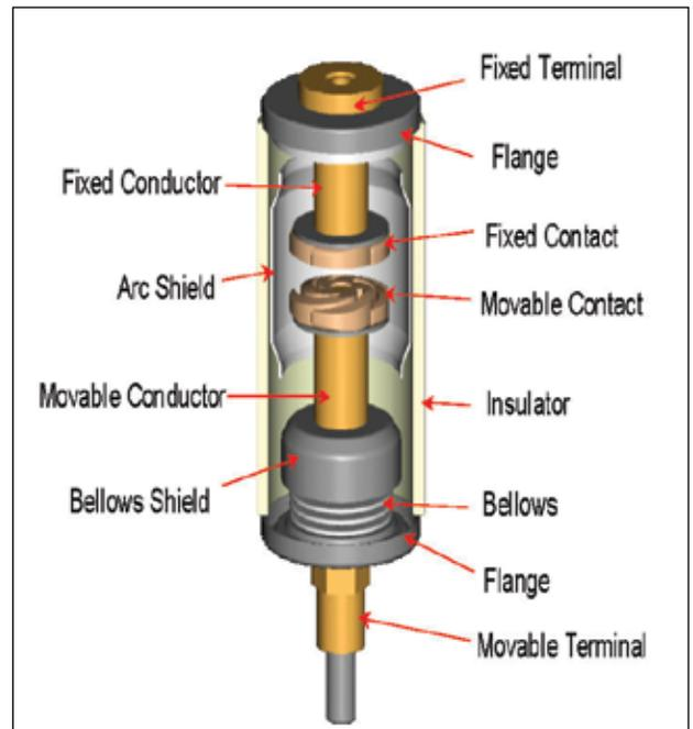
Figure 3 — Basic Structure of a Vacuum Interrupter
