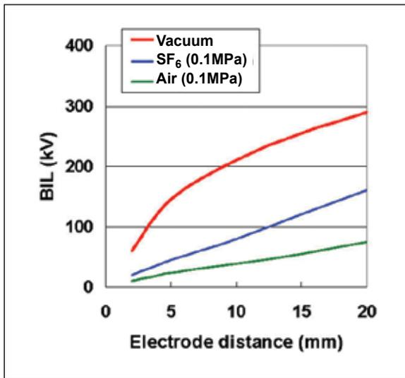
Figure 2 — Dielectric Strength Properties of Vacuum
