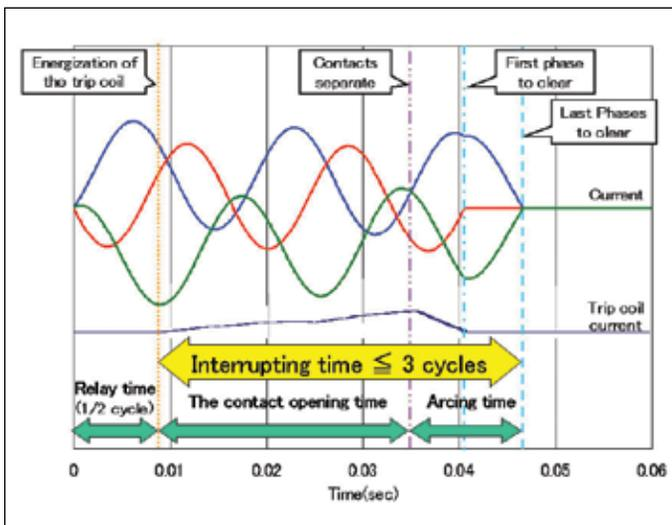
Figure 7 — Three-Phase Current Interruption for Three-Cycle CB
