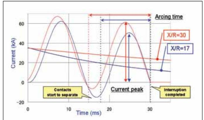
Figure 8 — Short Circuit Asymmetric Current (for 25 kA)
