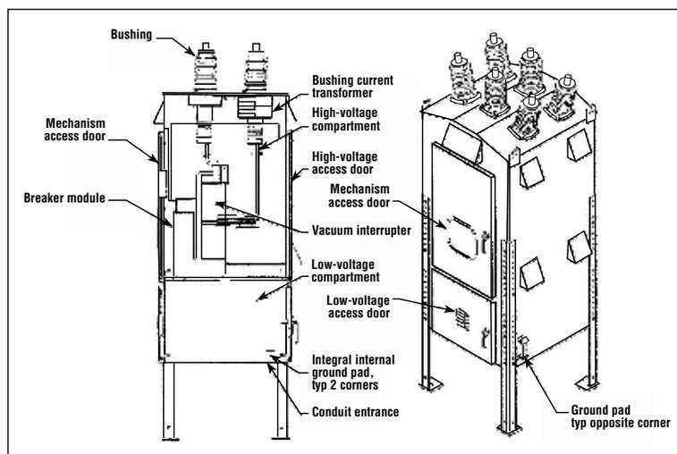
Figure 1 — Structure of an Outdoor VCB (17.5 kV-25 kA)
