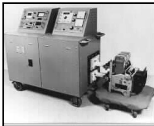
The EIL BTS-1000 used a multi-stage output transformer with series/parallel connections. It could produce over 100,000 amperes into a short circuit, and was capable of testing the largest circuit breakers in general use.
