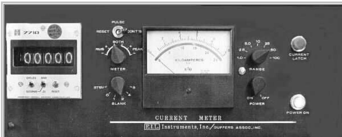
The "Duffers" Memory Ammeter, used in many EIL circuit breaker test sets, incorporated peak reading circuitry, and used blanking to reduce error from DC offset. It was soon replaced by the Accu-Amp, which used a true-RMS converter IC in conjunction with a fast-attack, slow decay circuit.
