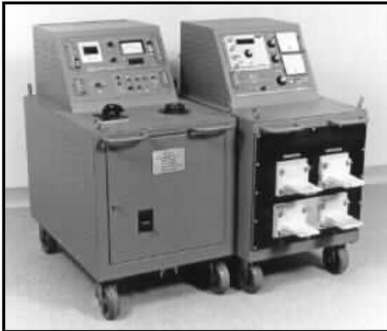
The 50,000 amp EIL BTS-500S was the top of the line for many years. It used a single E-I output transformer and tapped input autotransformer. Many are still in use today.
