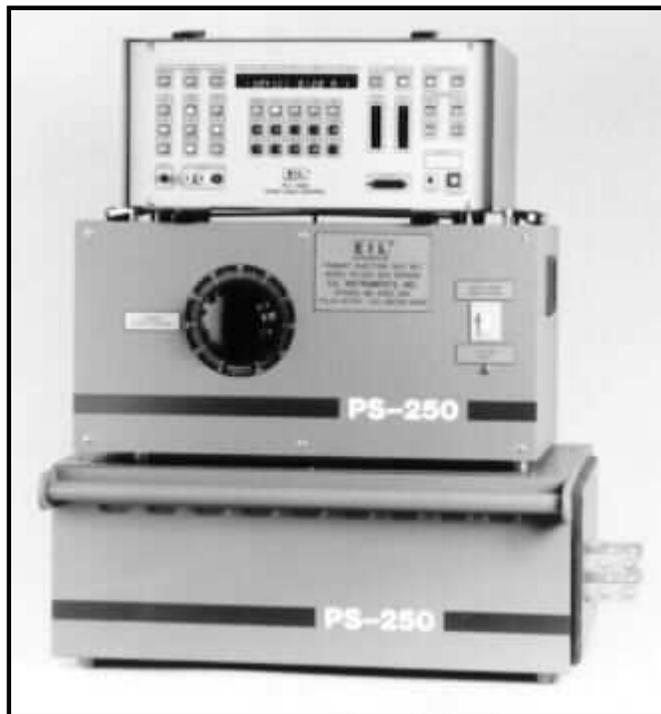
The EIL PS-250 was one of the first breaker test sets to use a microprocessor, but it retained some of the original analog signal preprocessing. Its major advantages were programmable auto-jog and current hold, and data storage, retrieval, and report printing.
