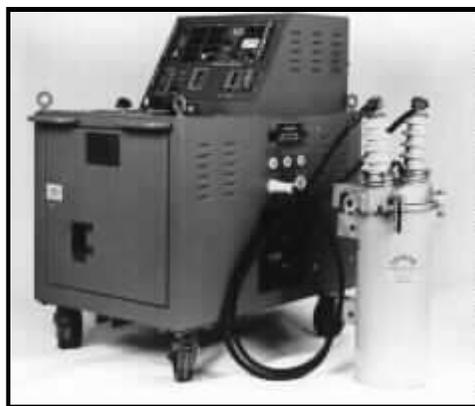
This is an EIL ORT-560 Recloser Test Set, with a typical recloser. The test set uses resistors to regulate the output current.
