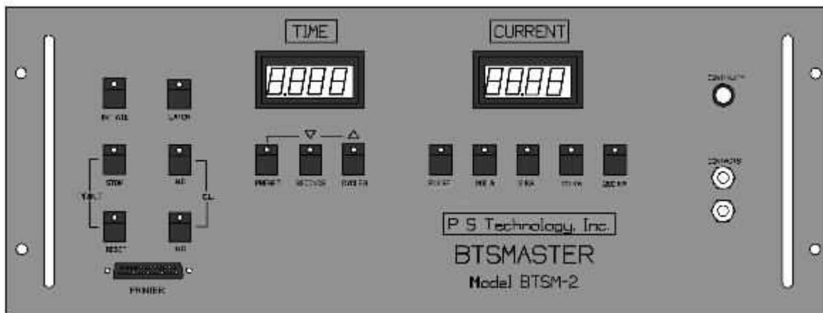
The BTSMaster, P S Technology's latest breaker testing instrument, incorporates an A/D converter and microprocessor for true-RMS reading of current, accurate reading of trip times, and a convenient programmable on time feature for auto-jog operation.
